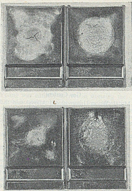
FIGS. A AND B.—Samples of D.T.D.424 Alloy Cast in the "Shrinkage-test" Die, showing the Effect of Gas Content; (above) De-gassed, and (below) Gassed.
