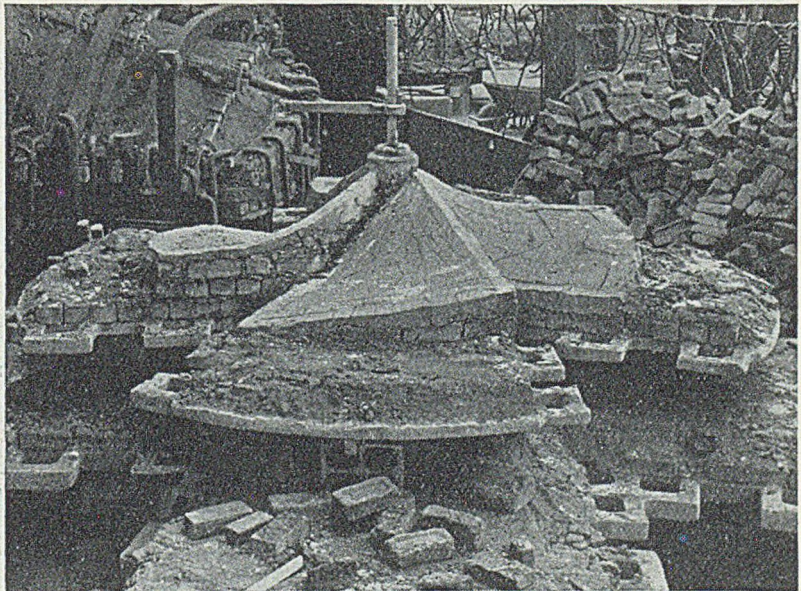
FIG. 1.—Drag Part of a Loam Mould for a Small Propeller Casting.
