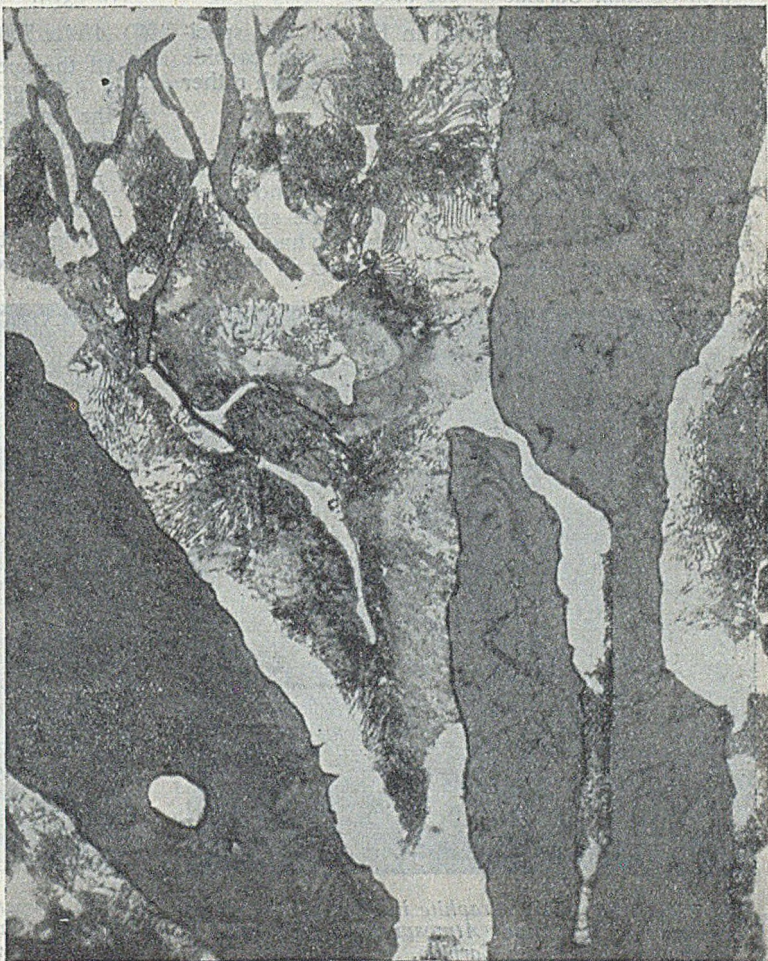
FIG. 5.—Coarse Hyper-eutectic Flake Graphite in a Matrix of Mixed Ferrite and Pearlite; Vacuum-melted Iron. \times 600 mags.
