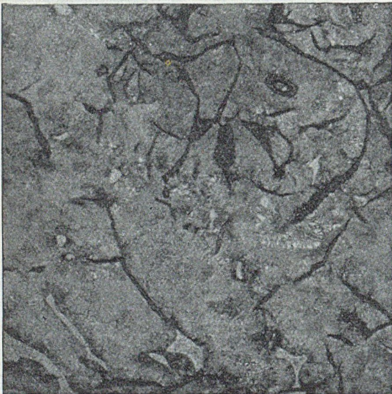
FIG. 7.—Medium-flake Graphite in Pearlite. Specimen Melted in Hydrogen Atmosphere at 750 mm. in contact with Calcium Carbide. \times 600 mags.
