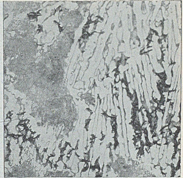
FIG. 11.—Central Zone of "Internal Chill" found in same Specimen as in Fig. 10. \times 600 mags.
