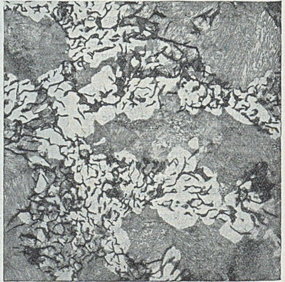
FIG. 9.—Supercooled Graphite and Ferrite in Pearlite Matrix. Specimen Melted in Nitrogen at 10 mm. in contact with Calcium Carbide. \times 600 mags.
