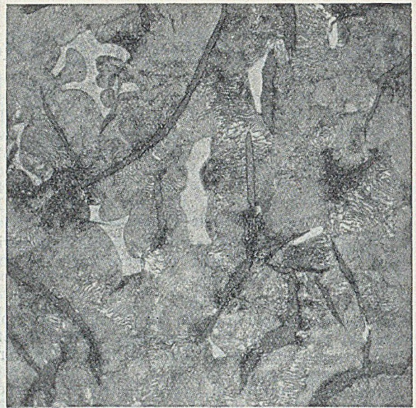
FIG. 8.—Grey-iron Structure of Specimen Melted in contact with Graphite in an Atmosphere of 10 mm. Nitrogen. \times 600 mags.
