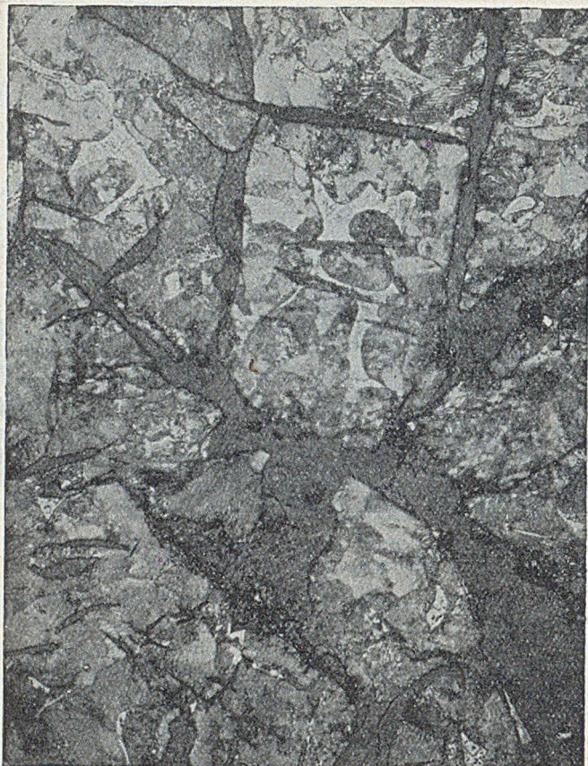
FIG. 12.—Largely Pearlitic Structure of Specimen Melted in Air at 750 mm. in contact with Lime. \times 600 mags.
