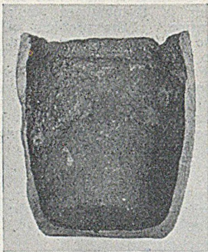
FIG. 1.—Cross-section of a Graphite Crucible which failed because of Thinning where the Furnace Flames impinged; the wall has spalled and is now only a Small Fraction of its Original Thickness.
