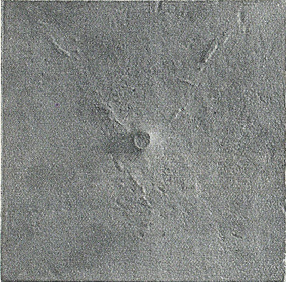
FIG. 11.—Surface of a Test-plate Casting made in Sand with 2.5 per cent. Coal-dust as well as 1.0 per cent. Wood-flour.
