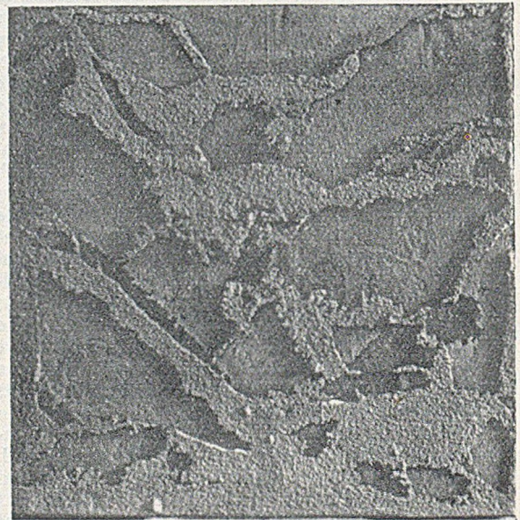
FIG. 7.—Test-plate cast in 60 secs. at 1,290 deg. C., in Sand containing 2.5 per cent. Coal-dust.
