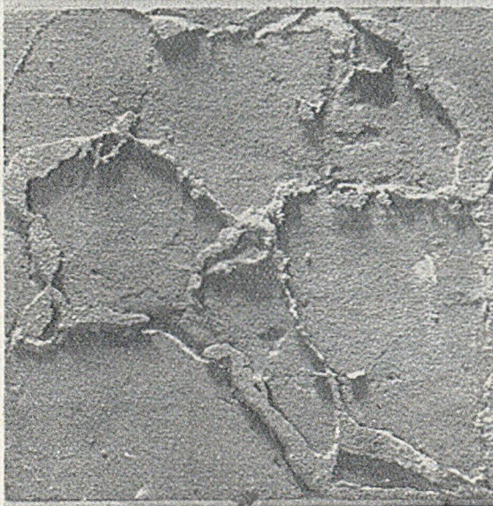
FIG. 6.—Top Surface of Thick Test-plate (see Fig. 3) cast in Ordinary Sand without Coal-dust.
