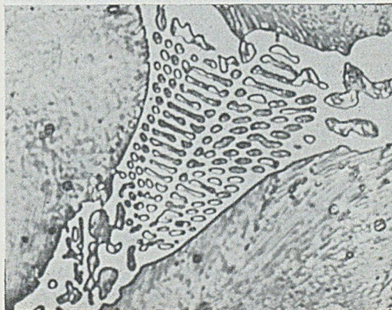
FIGS. 14 TO 16.—Occurrence and Influence of Phosphorus in Grey Cast Iron:—
