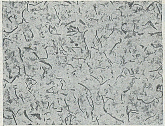
FIG. 9.—Iron of Similar Type to that shown in Fig. 8, but taken After Inoculation.
