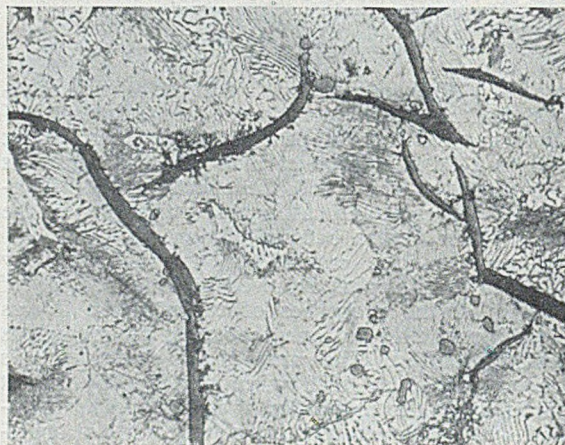
FIGS. 10 TO 13.—Occurrence of Sulphur in Cast Iron; FIG. 10 (TOP LEFT) Duplex Iron/Manganese-sulphide Inclusions; FIG. 11 (BOTTOM LEFT) Normal Angular-type MnS Inclusion; FIG. 12 (TOP RIGHT) Anchor-type MnS Inclusion; and FIG. 13 (BOTTOM RIGHT) Distribution of MnS in Inoculated Iron. Photomicrographs Figs. 10 to 12, all \times 1,000 , unetched. Fig. 13, \times 500 , etched in 4 per cent. Picral.
