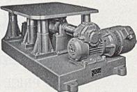
Patent Jolt Moulding machine eliminates hand ramming.
