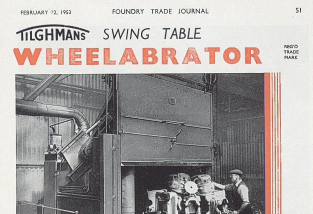
Equally suitable for cleaning castings weighing only a few pounds or up to two tons. The Swing Table is made in five sizes: 4ft. 6in., 6ft., 7ft. 6in., 9ft. and 10ft. diameter, with either one or two tables.
