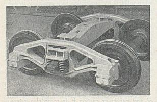
FIG. 6.—Side Frame and Bolster Assembly to form a Complete Bogie. Note the Clean Lines when this is Produced with Castings.
