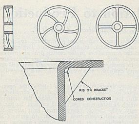
FIG. 1.—Coring of a Bracket Web and Re-design of Wheel Spokes to Eliminate Casting Stresses
