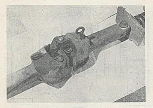
FIG. 5.—Design of Cast Steel Couplings as frequently used Abroad for Railway Rolling Stock and now to be adopted for British Railways.
