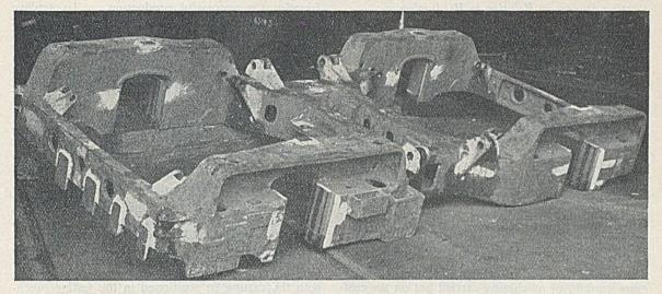
FIG. 7.—Cast-steel Bogic Frame which Replaced a Welded Assembly. It weighs 2 tons and has an average Metal Thickness of  $\frac{7}{5}$  in.
