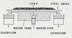
If you have difficulty with your warm sand adhering to patterns why not cool it on our patented water-cooled steel band conveyor as illustrated by diagrams above and on right.
