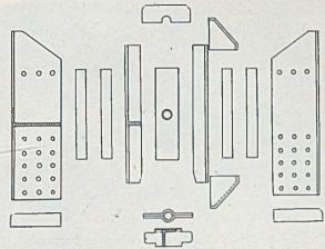
FIG. 4.—Seventeen Component Parts for a Centre Filler to be Fabricated by Welding.
