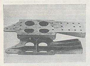
FIG. 3.—Three-piece Centre Filler Casting as now Produced for Railway Freight Car Manufacture.
