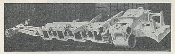
FIG. 8.—Cast-steel Locomotive Bed Typical of the Trend in America to make such Items (from 40 to 50 ft. long) as Castings. The Single Casting incorporates Cylinders and Cradle Frame.
