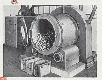
AIRLESS ROTARY BARREL BLAST CLEANING MACHINE
