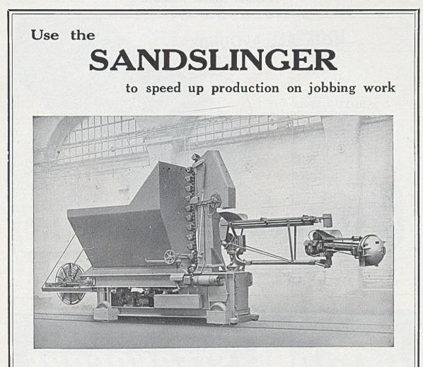
The Junior Motive Sandslinger, illustrated above, travels to and fro along a 3-ft. gauge track on both sides of which it provides a
