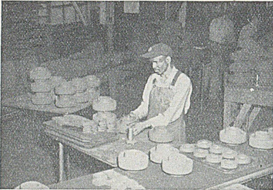
FIG. 15.—Performing the Finishing Operations on Cores taken from the Conveyor Belts.
