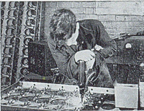
An electric stud-welding gun in operation on a dust collector component.
