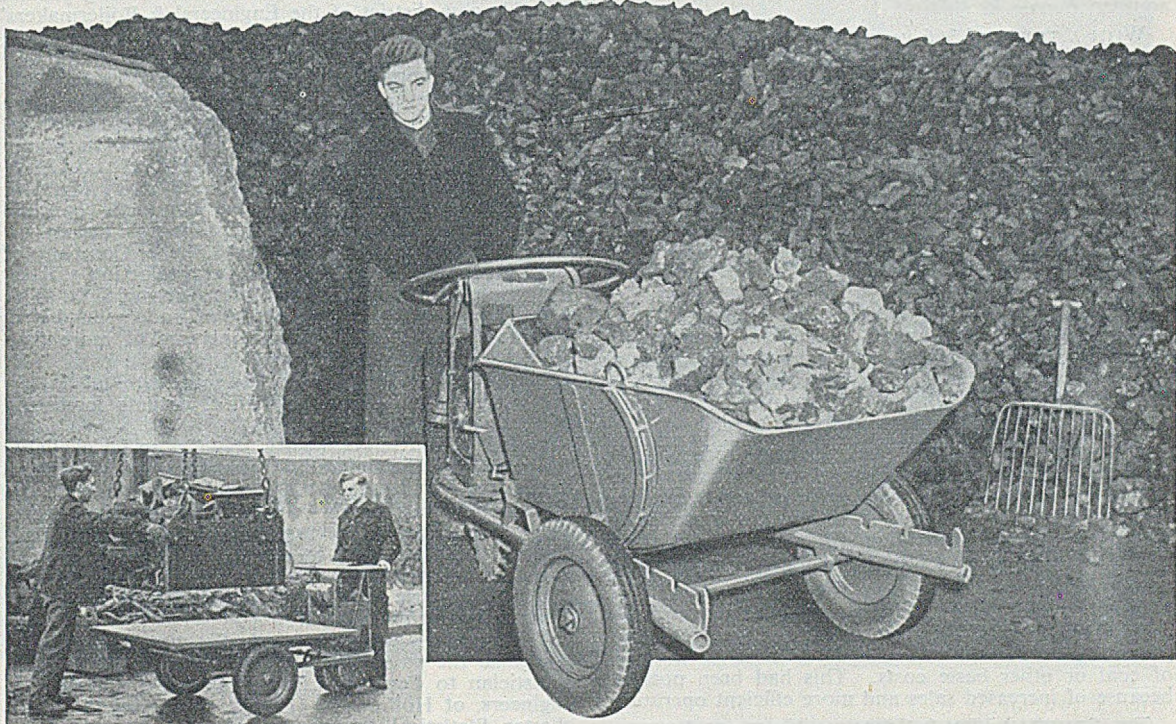
Loading scrap metal for cupola
