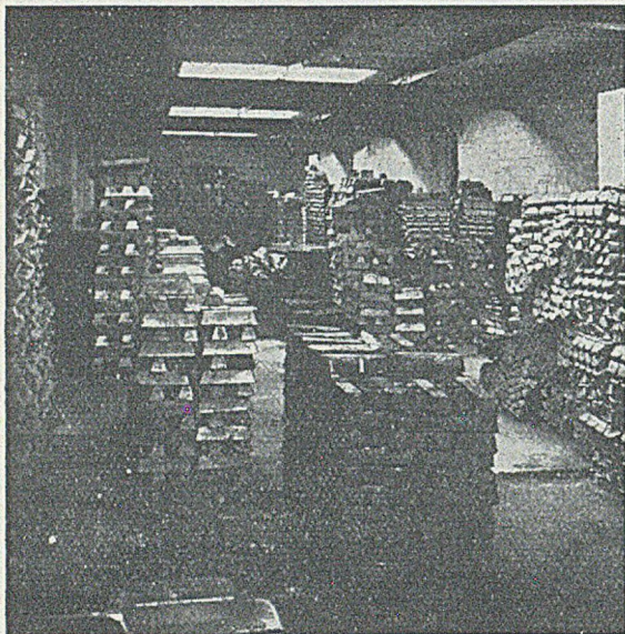
FIG. 5.—View of Stacked Non-ferrous Ingots in Part of the Metal Stores; Each Batch is kept separate according to Specification and All Scrap arising in the Works is similarly treated.
