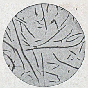
FLAKE GRAPHITE IRON (UNETCHED) x 100
