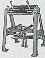
Hand Rammed Moulding Machines to turn-over and down-draw. Boxes up to 30in. x 18in. (standard 15in. x 15in.) can be handled.
