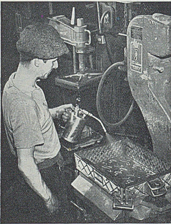
FIG. 1.—“Mysto” Hand-operated Pattern Sprayer in use at Shaw Foundry, Willenhall. (Note also the use of Slip Flasks on these Moulding Machines.)
