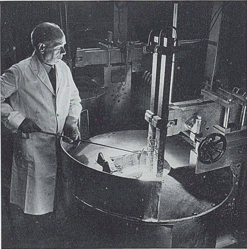
An electrically heated salt bath in the tool room: The Rover Co. Ltd., Birmingham
