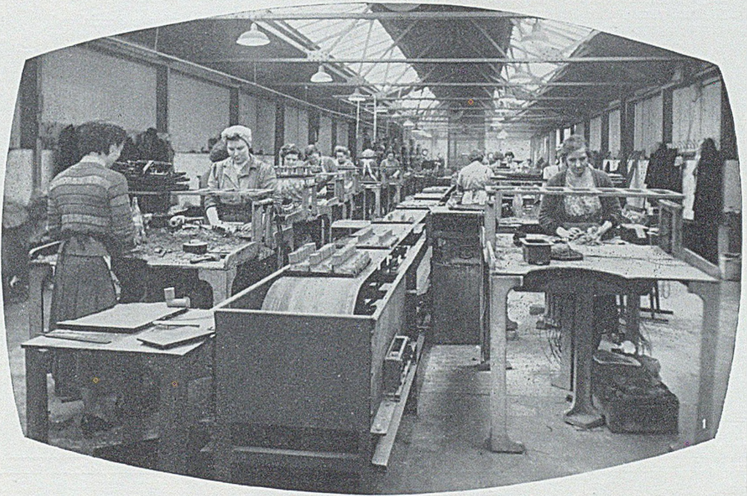
This photograph shows one of our many conveyors conveying cores from the benches to the drying stove.
