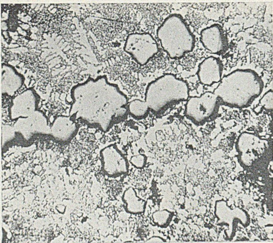
FIG. 4.—( \times 90 ) Chill-cast Alloy treated with 1 per cent. Sodium. Large, rounded Silicon Crystals. (Compare with Fig. 5.)
