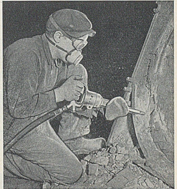
Above: One of the R Series Chipping Hammers, also employed at The Bofors Steel Works
