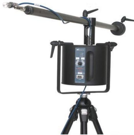
Fig. 29.1. Nor265 rotary boom by Norsonic [1]
