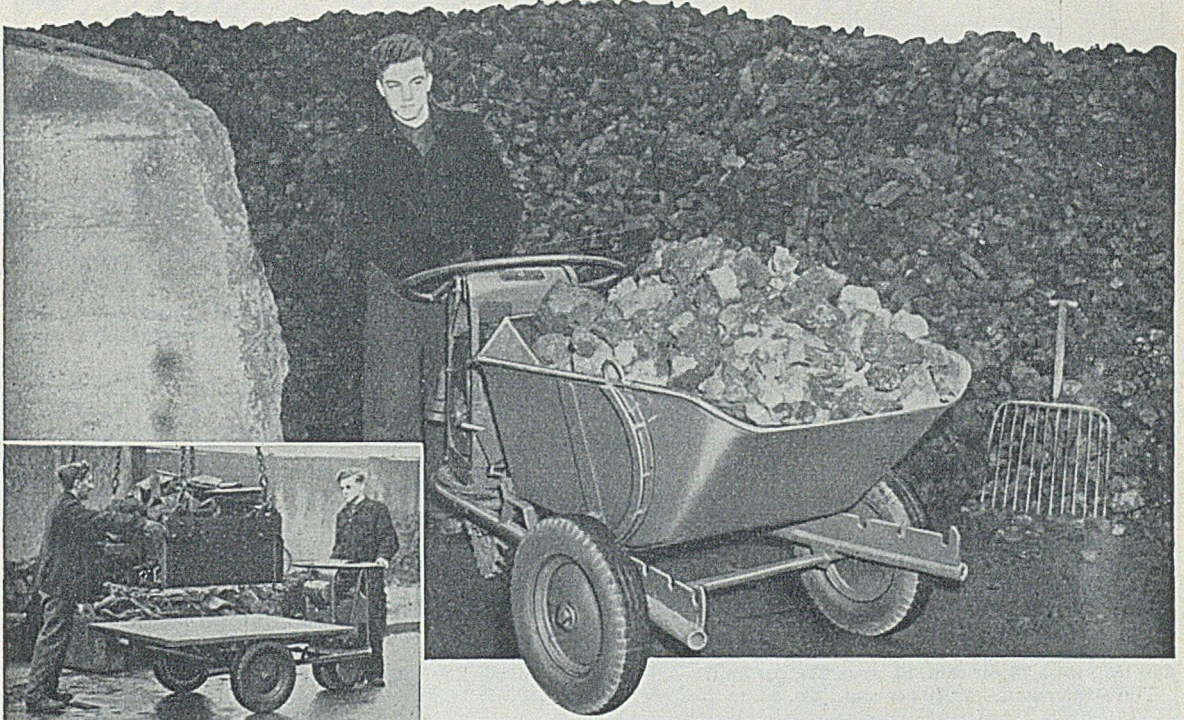
Loading scrap metal for cupola
