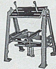
Hand Rammed Moulding Machines to turn-over and down-draw. Boxes up to 30in. x 18in. (standard 15in. x 15in.) can be handled.
