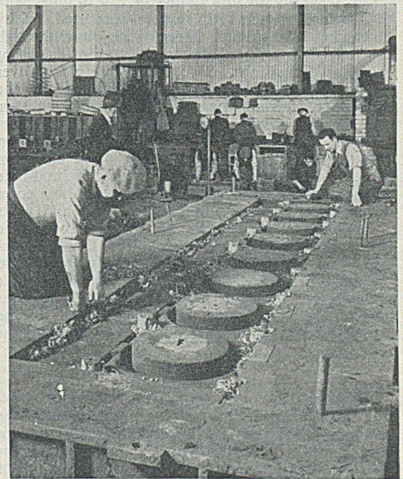
FIG. 10.—Cylinder-block Mould, at an Advanced Stage in Assembly, showing the Plugging of Spaces with Cotton Waste to Retain any Loose Sand.
