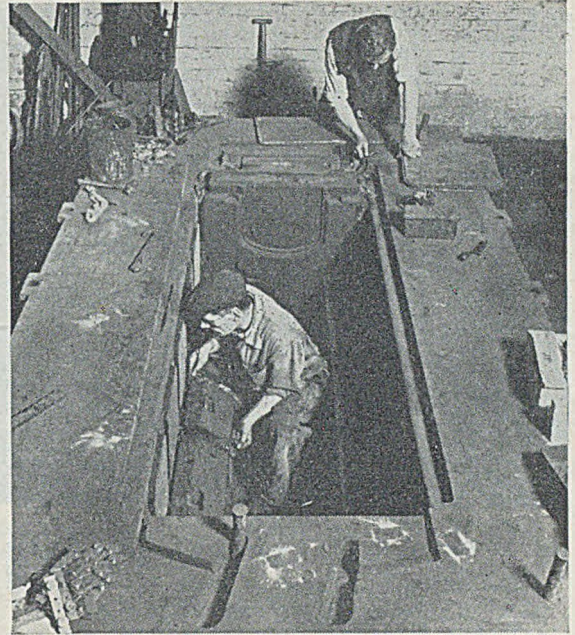
FIG. 5.—Coremaker preparing the Vents from the Mud-hole Cores of the Frame Castings.
