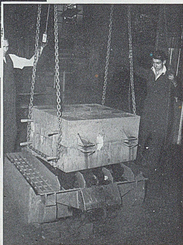
Dry Sand Mould weighing 1½ tons being rapidly knocked out on 4ft. 0in. square machine.
