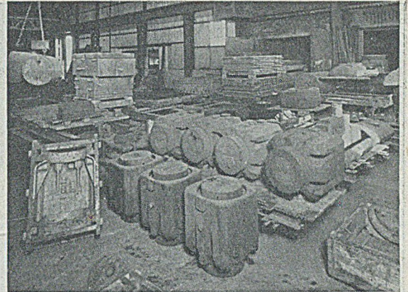
FIG. 9.—Group of Cores for the Cylinder-block Casting, the Seven Barrel Cores are prominently displayed.
