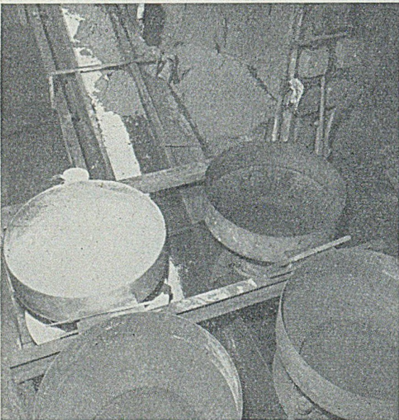
FIG. 13.—Arrangement of Four "Addition" Hoppers over Sand Conveyor Belt leading to the Measuring Hopper supplying the Batch-type Sand Mills.
