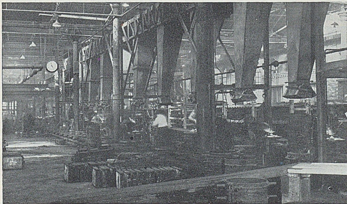
FIG. 11.—View of Platt Bros.' Mechanized Moulding Plant showing Ten Orthodox Jolt-squeeze Pin-lift Moulding Machines, Two Pairs of which have since been replaced by "Automold" arrangements.
