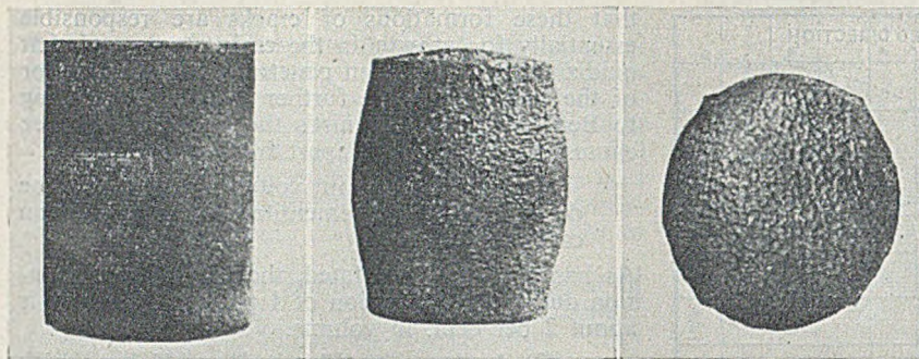
FIG. 3.—Steel Cylinder after Repeated Quenching, left to right: (a) Original; (b) after 200 Quenchings; (c) after 800 Quenchings. (Whiteley. 11 )
