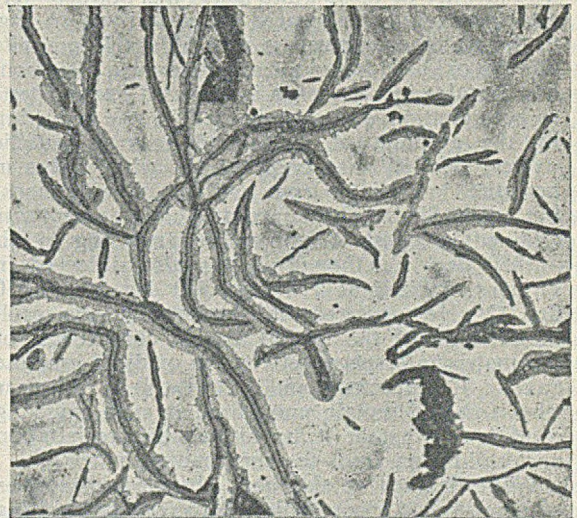
FIG. 7.—Ingot-mould Iron No. 4 after 60 days at 500 deg. C. in Air. Edge of specimen, \times 60 ; etched in 4 per cent. Picric and Ammonium Persulphate.
