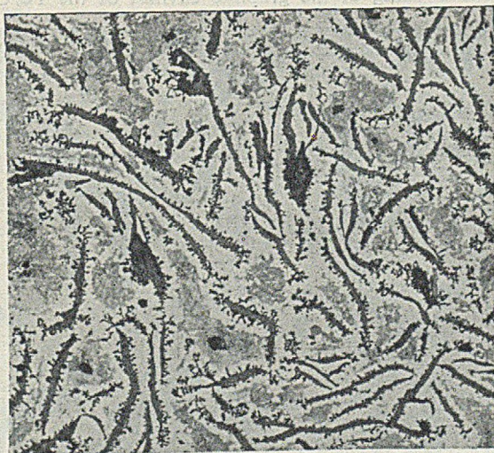
FIG. 10.—Specimen 3C2. Ingot-mould Iron No. 3, As-cast, after 100 heatings 650-900-650 deg. C. in Vacuum, showing 21.3 per cent. volume Growth; \times 60 ; etched in 4 per cent. Picral.
