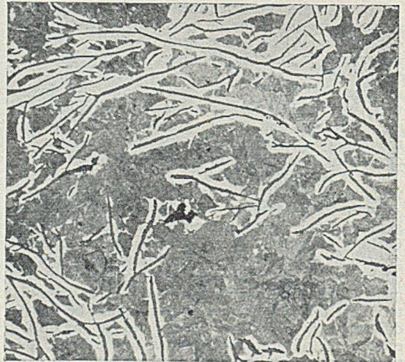
FIG. 23.—Ingot-mould Iron No. 3, Annealed 400 hrs. at 700 deg. C. in Vacuum, and then 16 hrs. at 930 deg. C. and Air-cooled (compare with Fig. 22); \times 60 ; etched in 4 per cent. Picral.
