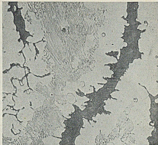
FIG. 11.—Specimen 3C2; same as Fig. 10, but \times 600 ; etched in 4 per cent. Picral.
