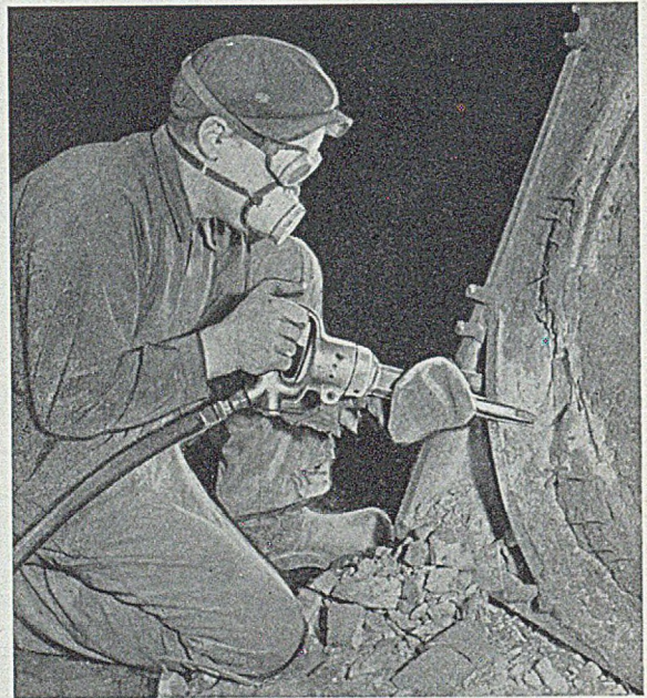
Above: One of the R Series Chipping Hammers, also employed at The Bofors Steel Works
