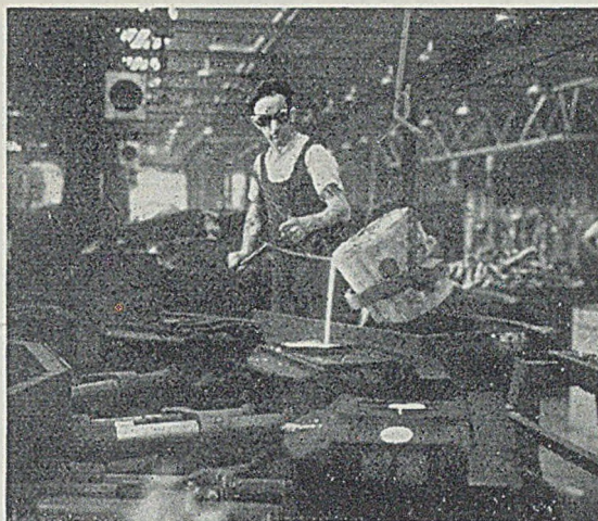
FIG. 5.—Close-up of Pouring on One of the Rotary Permanent-mould Machines in the Qualcast Foundries.
