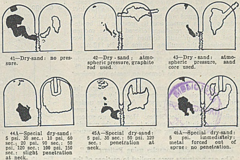
FIG. 17.—Sketches of Transverse Radiographs of "E" Design. Solid Black Areas show Shrinkage in the Casting. Outlined Areas show Shrinkage in the Riser.
