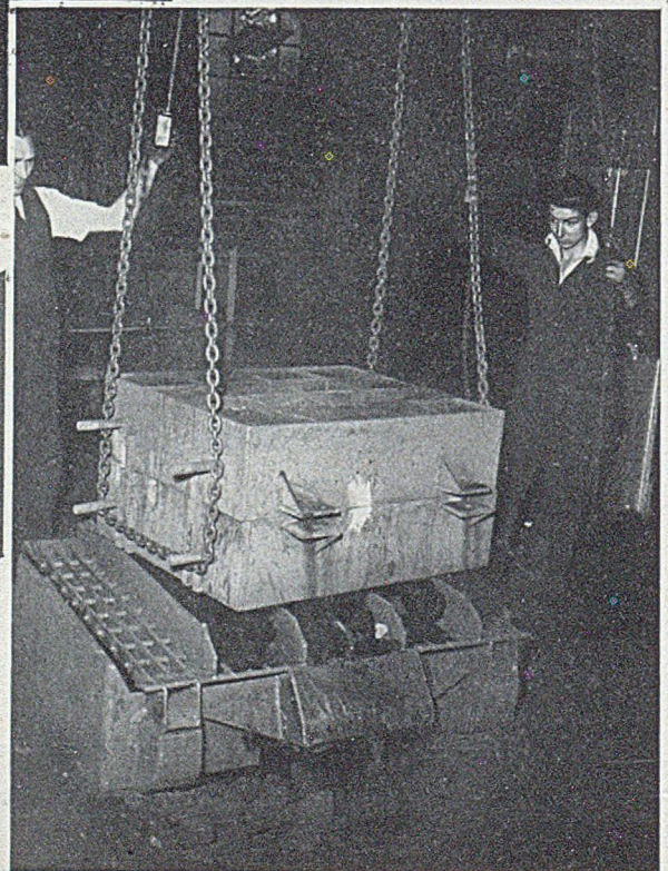
Dry Sand Mould weighing 1½ tons being rapidly knocked out on 4ft. 0in. square machine.
