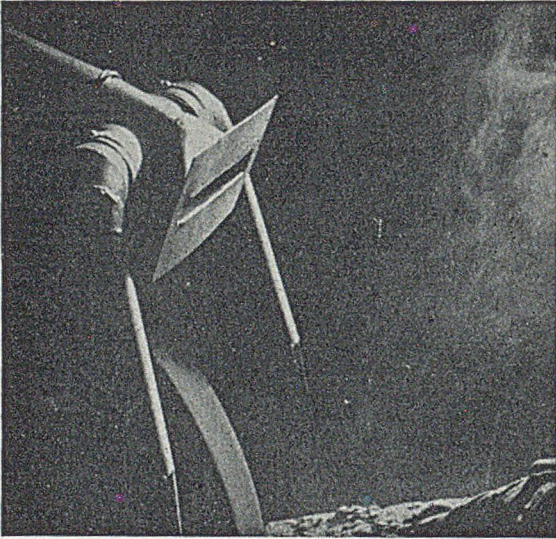
FIG. 4.—External System showing Dust rising past the Top Nozzle and moving up the Operator's Body to his Face (see line sketch, Fig. 3).
