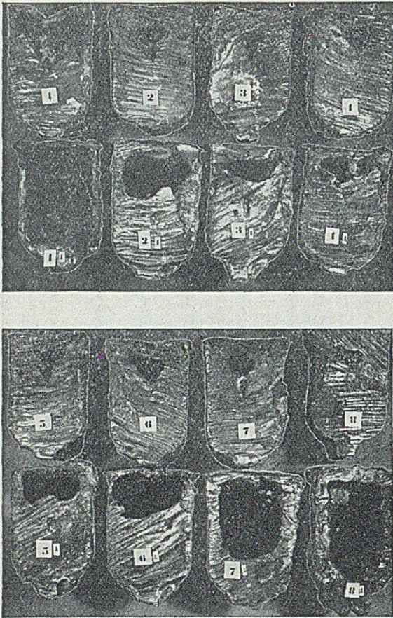
Fig. 5.—Sectioned Blind Top Risers of "A" Design, 1 to 8, without External Gas Pressure. 1A to 8A with External Gas Pressure.
