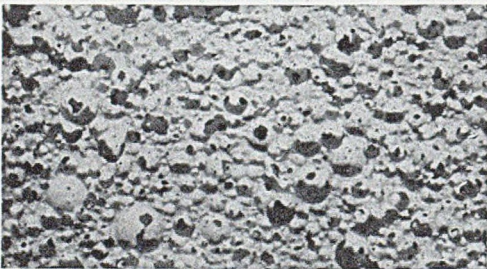
Intercommunicating cellular structure ensuring high permeability.
