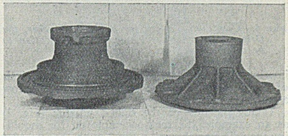
FIG. 2.—Hub Castings of Increased Design Complexity and, hence, Difficulty in Moulding.
