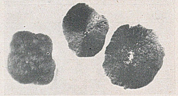
FIG. 5.—Section (7). Nodule I is being Totally removed. The White Spot in Nodule II has shrunk to a Point and Radial Pattern begins to appear. Nodule III shows Radial Structure near the Periphery.
