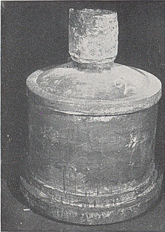
FIG. 13.—Sketch showing Running and Feeding Method for a Cylinder, using an Exothermic Sleeve; and FIG. 14, the Casting before removal of the Head.
