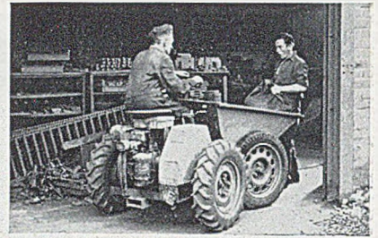
The hopper can be tipped even when it is turned at an angle of 35° to the chassis.
