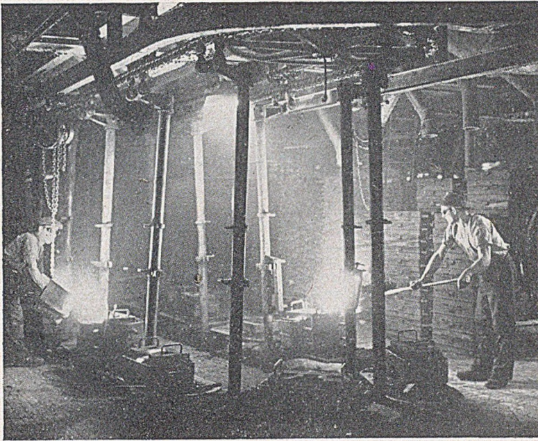
FIG. 6.—Pouring Medium-weight Castings on Pendulum Conveyors at the No. 4 Moulding Unit of Ford's, Dagenham.
