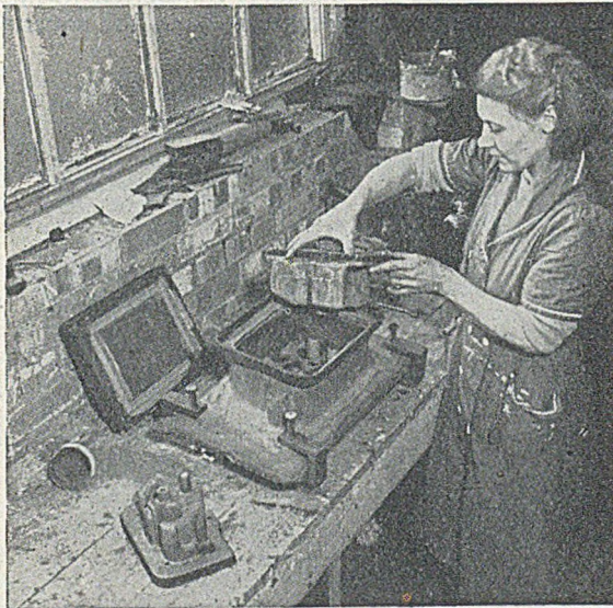
FIG. 13.—Assembly of the Mould Parts shown in Fig. 9. Note the D-shaped Clamps used to fix the Shells ready for casting.
