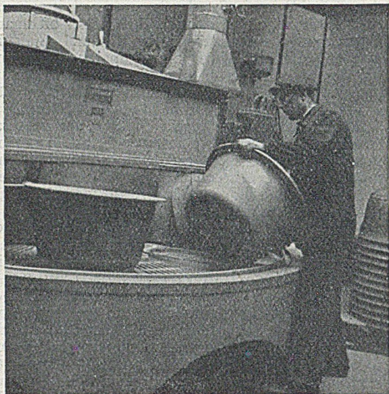
FIG. 9.—Large Cast-iron Pots for subsequent enamelling in White Finishes over Matt Ground-coat after being cleaned by Sandblasting.
