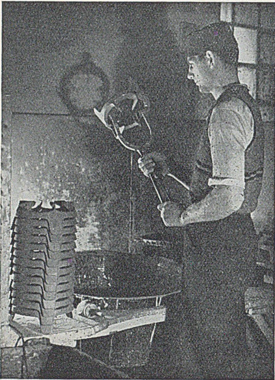
FIG. 4.—Portable Gas Rings being dipped in an Annealing-type Ground-coat by the use of Tongs.
