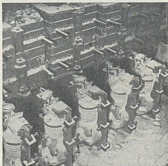
FIG. 23.—Group of Moulds shown in Fig. 22 after standing for about 10 min. following Pouring. Note the decrepitation of the Shell Bodies, leaving the Edges and Clamps standing.
