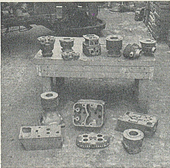
FIGS. 1 TO 3.—Groups of Typical Air-cooled Cylinder and Diesel-engine Head Castings made by the Author's Company in Shell Moulds. Many Jobs were previously made by Block Core Methods.
