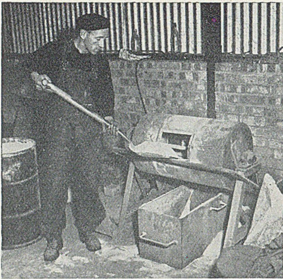
FIG. 4.—Simple Mixer for Resin/Sand for Shell Moulding. It is equipped with Internal Vanes and driven at 25 r.p.m. by a 1 h.p. Motor.
