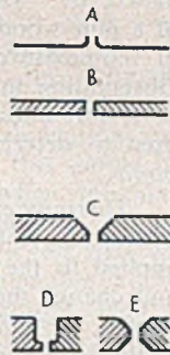
Fig. 4.—Various methods for preparing weld edges. (See column 3 of Table 1.)
