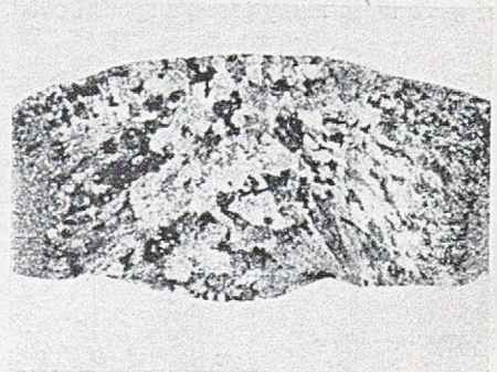
Fig. 94.—Macro-structure of cross-section of unheat-treated arc weld in Avional M. (See also Fig. 93.)
