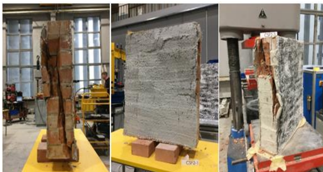
Fot. 5.1.4-3. Zniszczone elementy próbne dwustronnie wzmocnione serii CSF2 po badaniu Photos 5.1.4-3. Destroyed bilateral reinforced test pieces of the CSF2 series after testing
