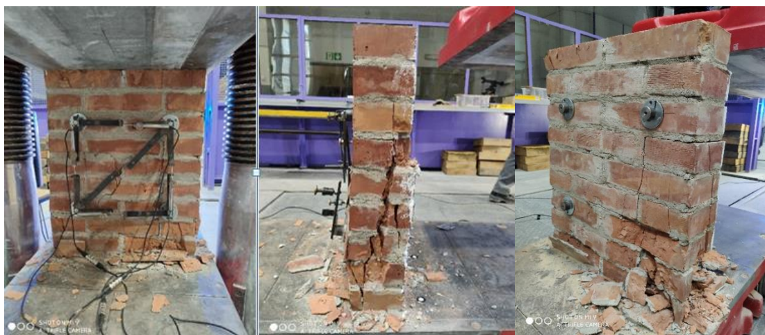
Fot. 5.1.4-1. Elementy próbne serii CS po badaniu Photos 5.1.4-1. CS series test pieces after testing
