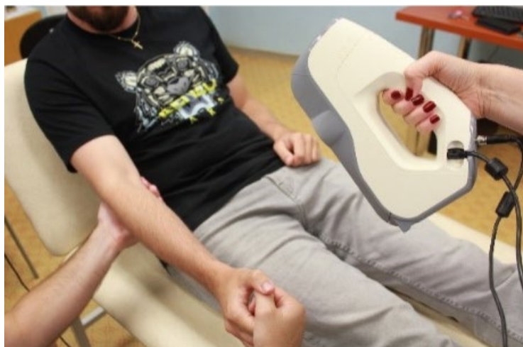
Fig. 16. Scanning of the hand and forearm using an assistant [25]
