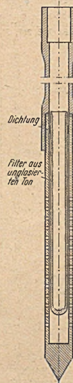
Bild 13. Meßbohrspitze für Porenwasserdruckmessungen in organischen Böden (entnommen aus Cuperus-de Nie, Strengthening the roadbed of a railway, supported by soft soil and situated amidst the buildings of the central port of a town. Proc. Rotterdam 1948, Bd. II, S. 1)*.
