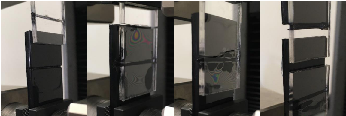
Fig. 9. Four types of failure observed, from left – on the weld, in the parent material, in the immediate vicinity of the weld and on the vapour channel
