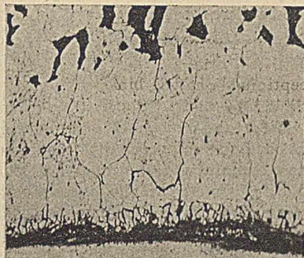
FIG. 4—STELLITE IN STEEL. X 100
