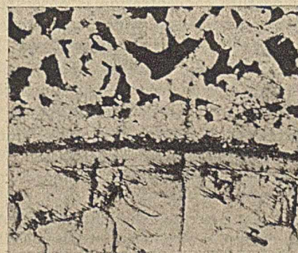
FIG. 7—ILLIUM IN CARBON STEEL. X 100
