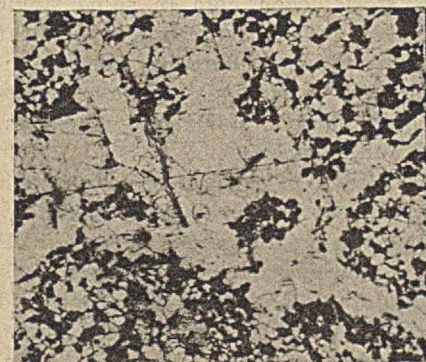
FIG. 10—TITANIUM STEEL WITH SEGREGATED FERRITE. X 100
