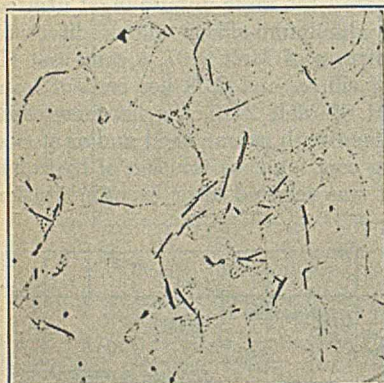
Figure 6—2.8 Si. \times 100 Sand-cast. 16,370-10.2-31. Still larger needles of X and increased quantity of Al-Si, often with fine needles of X
