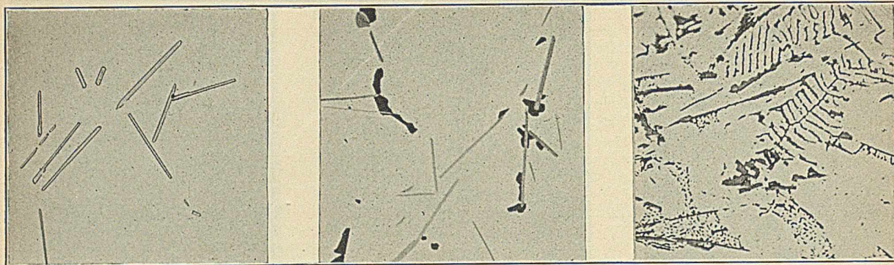
Figure 15—1.2 Si. \times 500 Quenched and aged. Needles of X. Si particles are in solution. Compare with Figure 13
