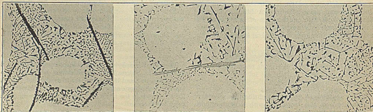
Figure 18—2.5 Si. \times 500 Sand-cast. Large needles of X cutting through Al-Si eutectic which contains fine needles of X. Note elongated Si particles
