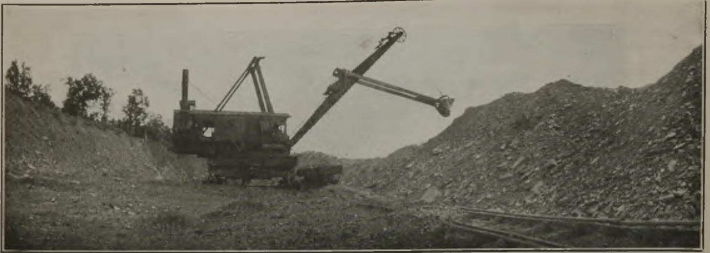
RIPPING THE OVERBURDEN FROM WESTERN KENTUCKY COAL WITH A MAMMOTH SHOVEL Most of the big shovels in the rapidly spreading stripping movement of that section of Kentucky are steam-operated. Central-station electric service is none too general yet. The cover on this coal varies at most strip plants between 25 and 35 ft., but in spots runs up as high as 50 ft. West Kentucky as a stripping field was only lately discovered.
