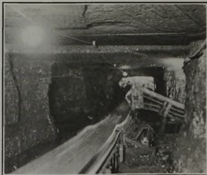
Fig. 8—Gallery Boom Feeds Lateral Conveyor
