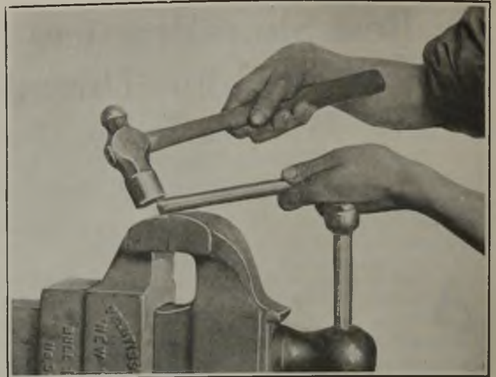
Fig. 5—Shaping Rod for Reception of Die
