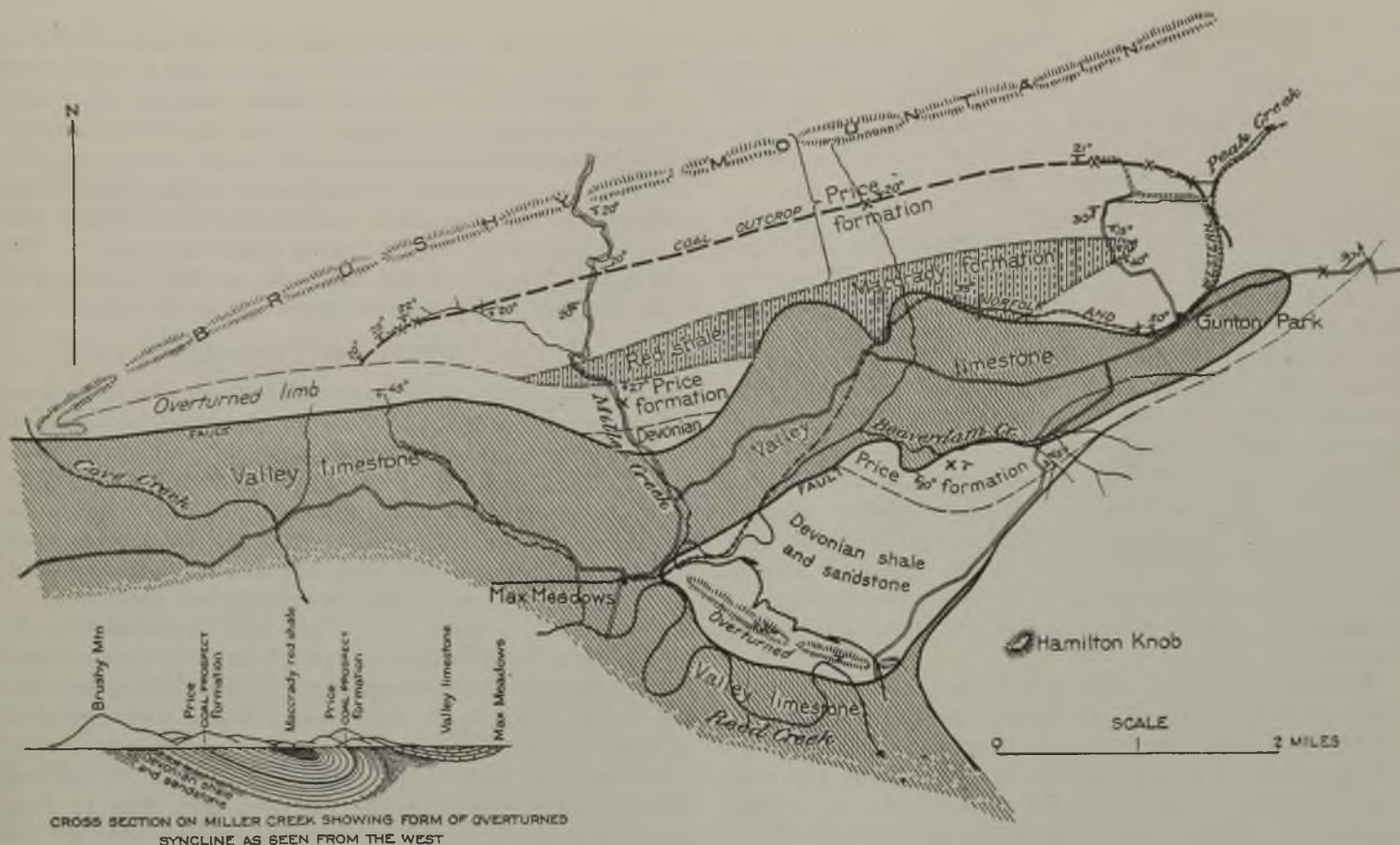
Fig. 3—Max Meadows Coal Field with Section Showing Form of Syncline
