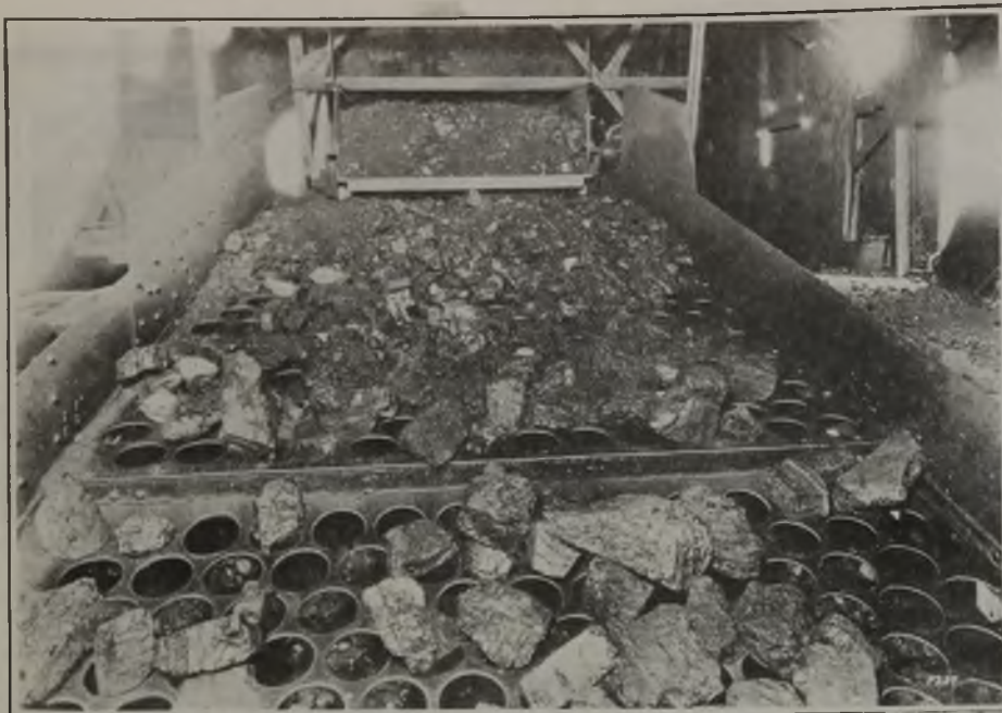
Fig. 1—Lump Screens in a Tippel
