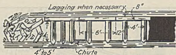
Fig. 7—How the Face Is Timbered
