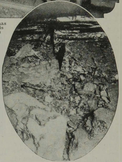
AFTER a shot in a center sheared face. The size of the coal produced speaks for itself.
