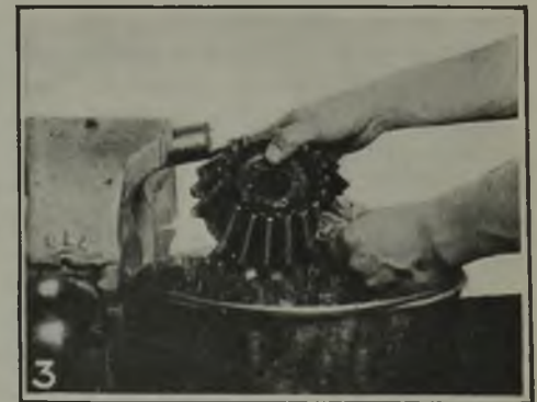
Fig. 3—Removing all Grease
