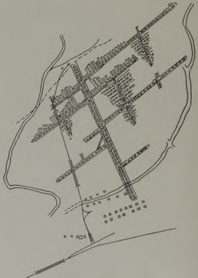
Fig. 16—Modification of Mining Used on Medium Pitches
