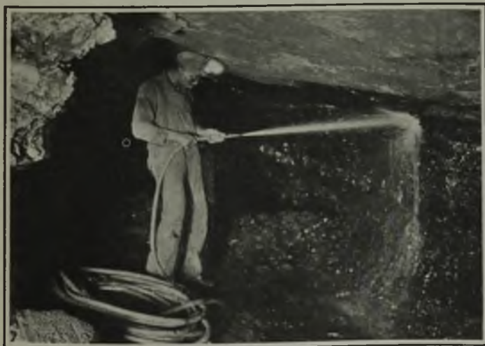
Fig. 26—Washing Down Ribs, Floor and Roof
