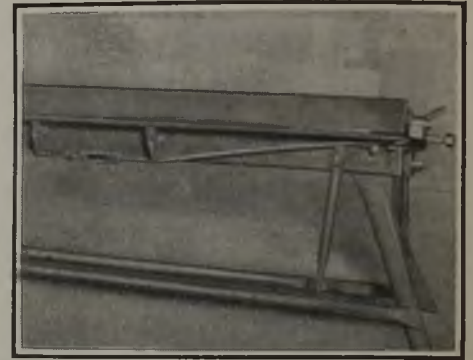
Fig. 2—Welded Parts for Bender
