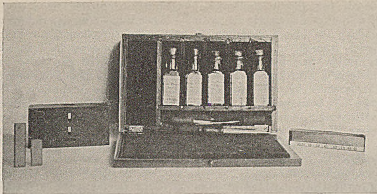
Above: Apparatus for Determining H-ion Concentration (Acidity or Alkalinity) of Mine Waters
