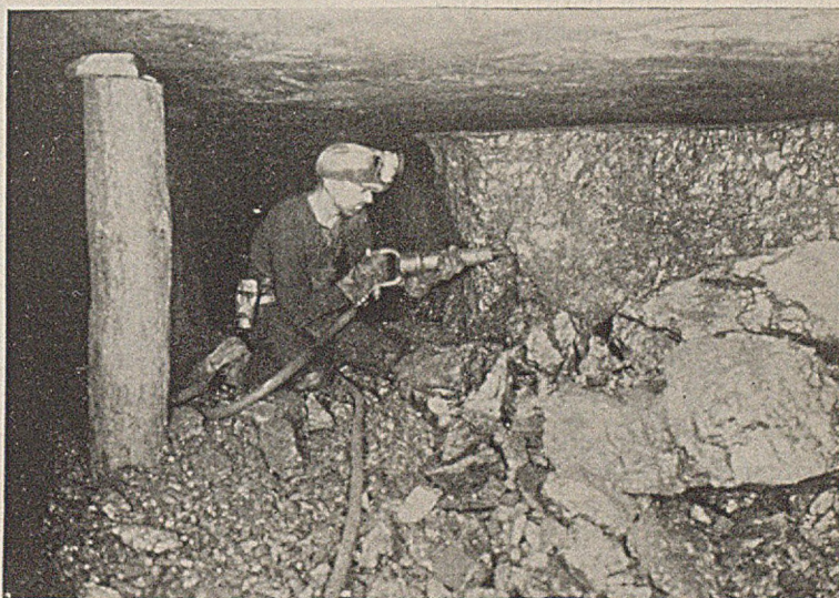
Using the Pneumatic Pick on a 300-Ft. Wall. Two Men Can Loosen Enough Coal to Keep Eleven or Twelve Loaders Busy
