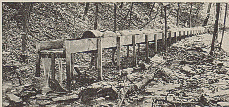
Experimental Flume Used in Testing Culverts With Acid Mine Water
