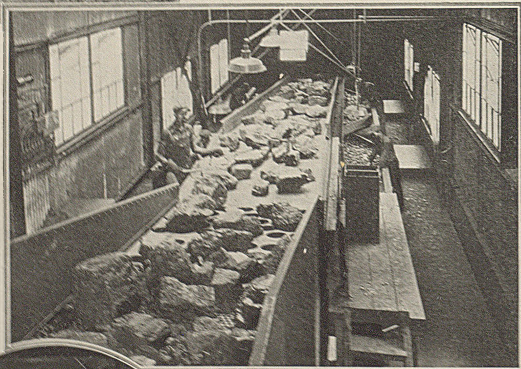
The Picking Table Screen Is Well Illuminated From Windows and Skylights
